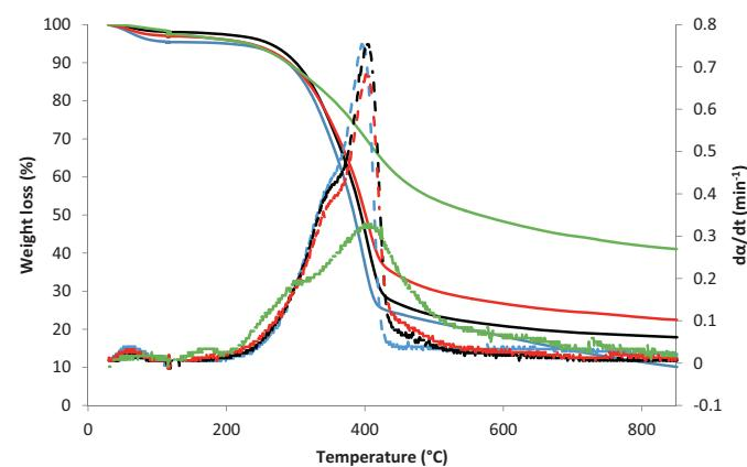
**Fig. 4.** Thermogravimetric and derivative curves for the raw materials (TGA —; DTG — · ) *Pinus Radiata* and Acetocell lignin (TGA —; DTG — · ) and the coated materials  $\text{Li}_{20}$  (TGA —; DTG — · ) and  $\text{Li}_{40}$  (TGA —; DTG — · ).
