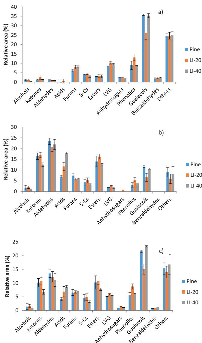
**Fig. 8.** Relative percentage of product distribution for (a) the BOC fraction, (b) the BOP fraction and (c) combined fractions.
