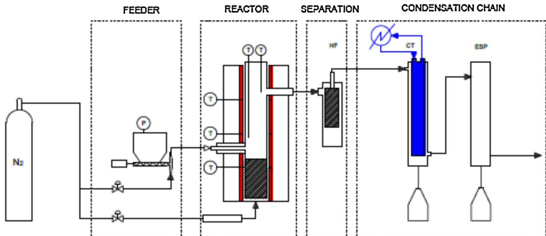
Fig. 1. Fast pyrolysis set-up showing the four sections.
