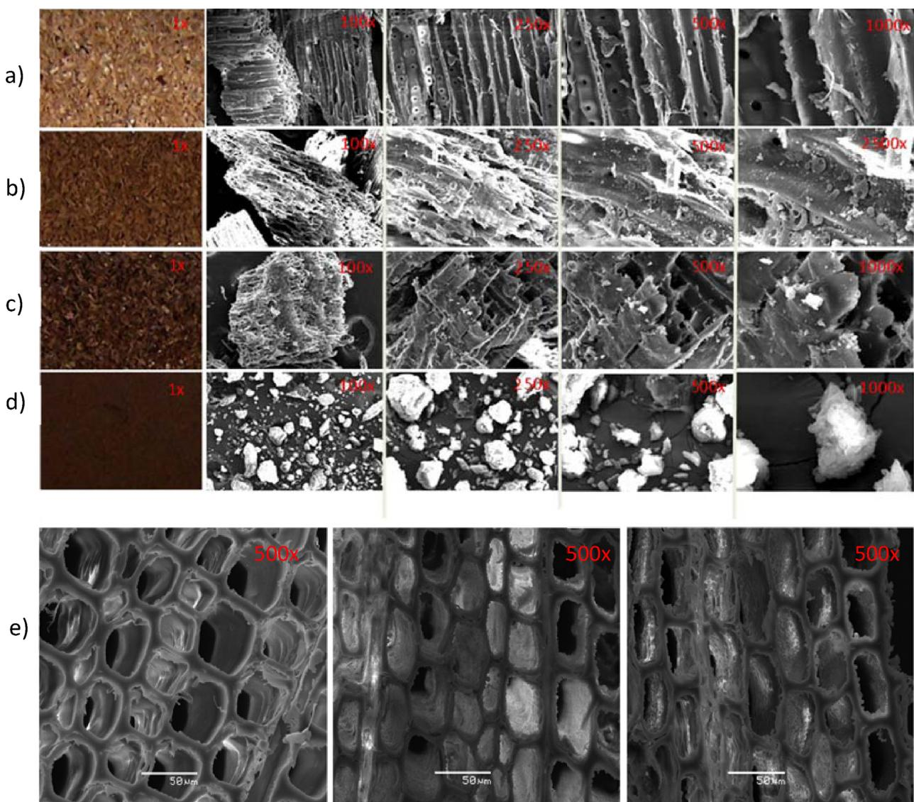
**Fig. 6.** SEM images of (a) Pine, (b) Li<sub>20</sub>, (c) Li<sub>40</sub>, (d) acid-extracted lignin powder and (e) pores of samples.
