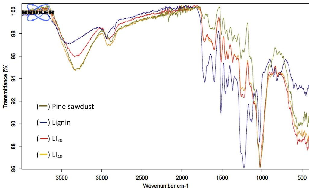
**Fig. 2.** ATR–FTIR spectra of raw and coated materials.
