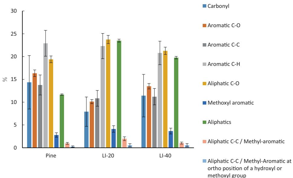
**Fig. 7.** Relative percentages of functional groups determined by  $^{13}\text{C}$  NMR for the BOP fraction.
