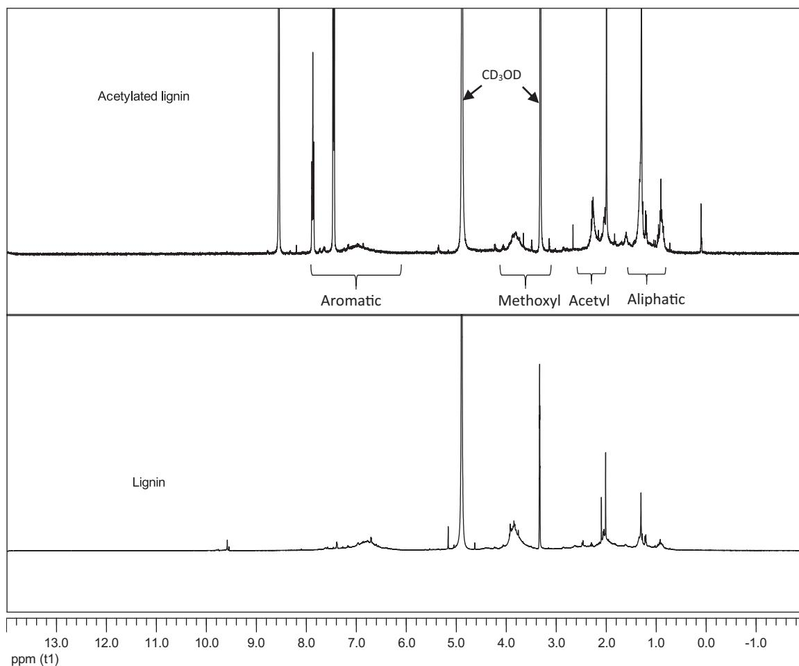
**Fig. 3.** <sup>1</sup>H NMR spectra of (a) the acetylated and (b) non-acetylated lignins with the following signal assignments: 10.0–9.7 ppm for H in benzaldehyde units, 8.0–6.0 ppm for aromatic H in sinapyl (S) and G units, 4.2–3.1 ppm for methoxyl H, 2.5–2.2 ppm for H in aromatic acetates, 2.2–1.9 for H in aliphatic acetates and 1.5–0.8 ppm for aliphatic H.
