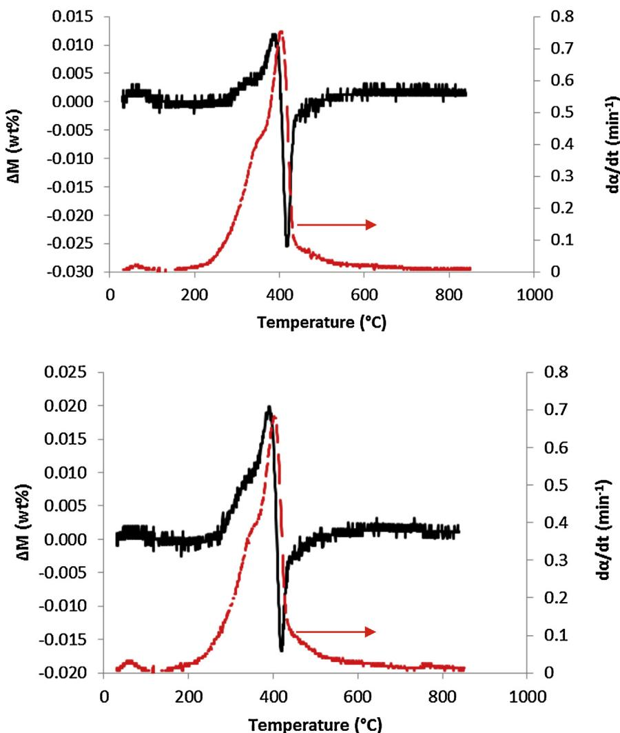
**Fig. 5.** Synergistic effect ( $\Delta M$ ) and derivated thermogravimetric curves ( $d\alpha/dt$ ) for (a)  $\text{Li}_{20}$  and (b)  $\text{Li}_{40}$  coated materials.
